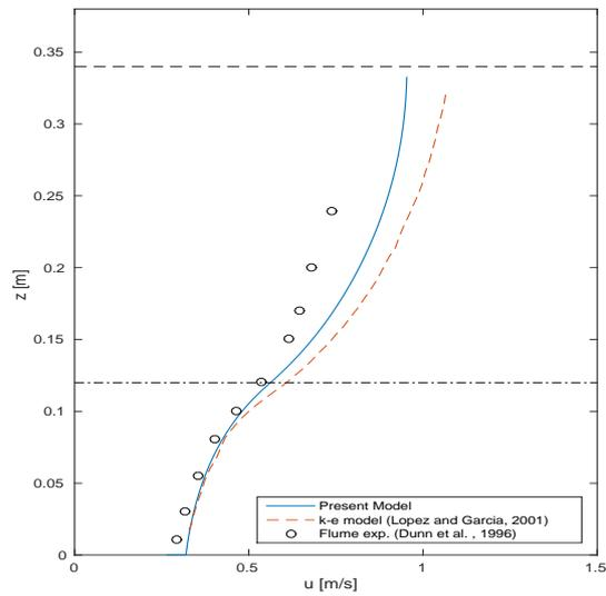
Figure 2: Comparison of the predicted velocity profile between the present  $k-\varepsilon$  model, the  $k-\varepsilon$  model from Lopez and Garcia (2001) and experimental data from Dunn et al. (1996). Here  $u$  is the spatially averaged mean velocity and  $z$  is the water depth. The horizontal dashed and dash-dot line indicate the water surface  $H$  and the canopy height  $h$ , respectively.
