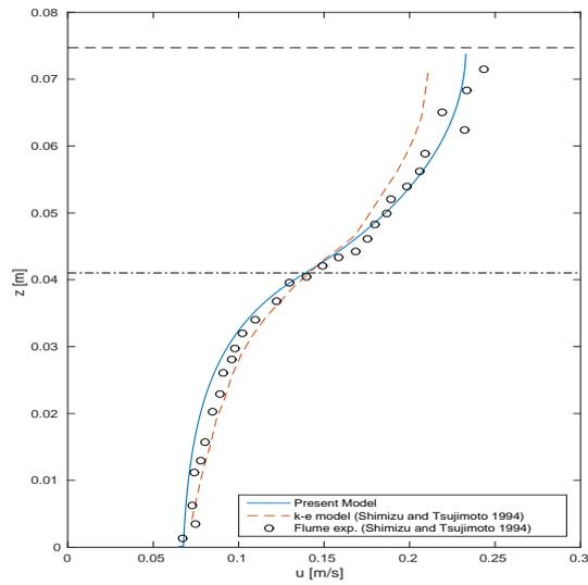
Figure 1: Comparison of the predicted velocity profile between the present  $k-\varepsilon$  model, the  $k-\varepsilon$  model and flume experiments from Shimizu and Tsujimoto (1994). Here  $u$  is the spatially averaged mean velocity and  $z$  is the water depth. The horizontal dashed and dash-dot line indicate the water surface  $H$  and canopy height  $h$ , respectively.
